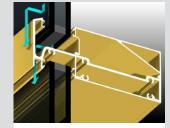
Concealed drainage designed to shed water more efficiently. Very high water performance greater than 600 Pa.
